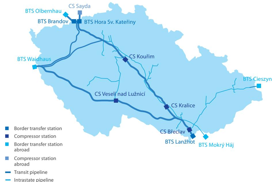
NET4GAS operates pipelines for the international transit and national transmission of natural gas with a total length of more than 3,800 km, with nominal diameters ranging from DN 80 to DN 1400 and nominal pressures ranging from 4.0 to 8.4 MPa.
