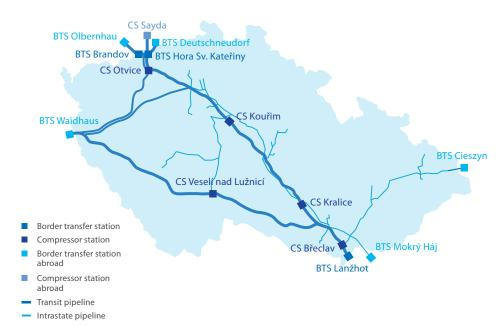
NET4GAS operates pipelines for the international transit and national transmission of natural gas with a total length of 3,973 km, with nominal diameters ranging from DN 80 to DN 1400 and nominal pressures ranging from 4.0 to 8.5 MPa.
